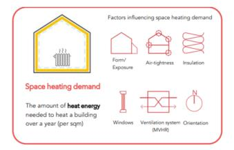
Energy Use Intensity (EUI) represents the total amount of energy used by a building divided by its floor area (GIA) and is reported in kWh/m2 year. The EUI is a good indicator of the energy efficiency of a home/building and can be calculated at both the design stage and post completion. For buildings heated by an individual heating system, performance monitoring will be simple as it will be the annual 'energy at the meter' divided by the floor area.
